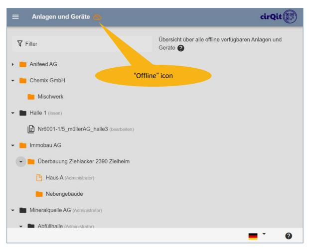
cirQit supports reading and editing circuit diagrams without network. Previously opened circuit diagrams are saved in the browser cache. These circuit diagrams are now also available offline. The application locally saves changes made during offline operation and uploads them to the cirQit Cloud when the availability of the network is restored.
